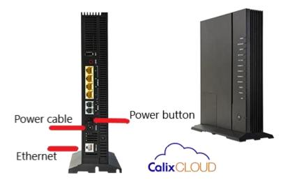
Step 3 – Once power and ethernet have been established, wait approximately 10 minutes for the new Blink router to download the correct Wifi information. When completed, the Blink router should be producing 2 wireless networks that correspond to the customers last name followed by "\_2.4" and "\_5ghz". The password will always be set to the word blink followed by the customer number which is part of the customer's account number with Barbourville Utilities.
